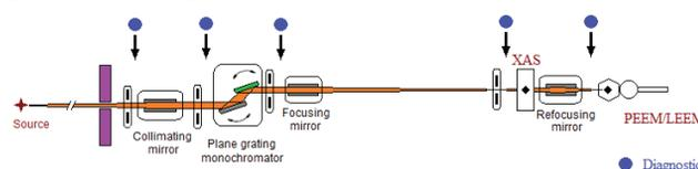
Figure 5: The conceptual layout of Solaris beamline.
